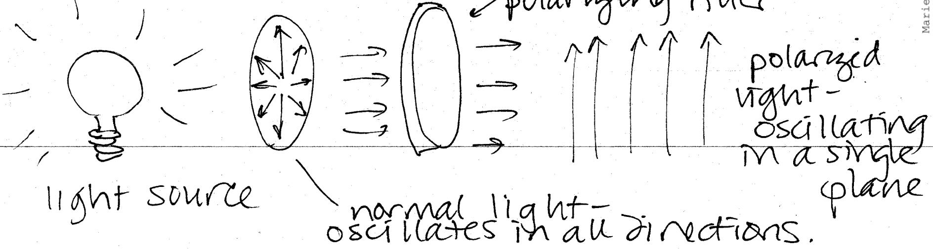
We use a polarimeter to measure optical rotation of a sample
