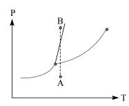
Which one of the following describes the sequence of phase changes that would occur when raising the pressure at constant temperature, as indicated by the dotted line from A to B?
