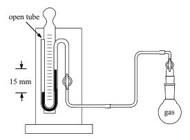
The mercury level in the outer arm is lower than the level of the inner arm by 15 mm. A barometer in the laboratory reads 756 mm Hg. What is the pressure of the gas sample in mm Hg?
